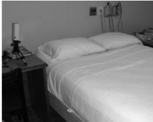
Εικόνα 10: Αισθητήρας κομοδίνου. P. Chazal, N. Fox, E. O'Hare, C. Heneghan, A. Zaffaroni, P. Boyle, S. Smith, C. O'Connell, W. T. McNicholas. Sleep/wake measurement using a non-contact biomotion sensor. 12 August 2010. https://doi.org/10.1111/j.1365-2869.2010.00876 .
