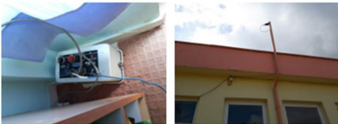
Figure 2.16 The SOUD SGM station, the REF TEK 130-SM and the GPS antenna
