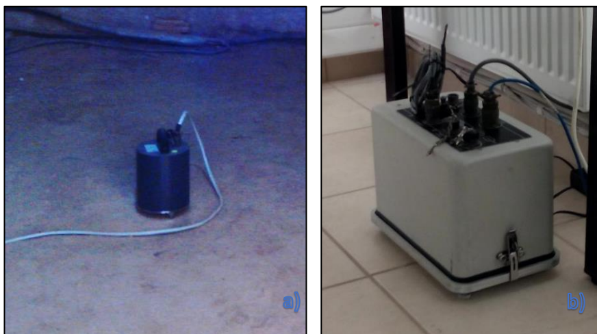
Figure 1.1. Some common used seismological sensors: a) broadband seismometer (Guralp 3ESPC - http://www.guralp.com/products/instruments/guralp-3-series ), b) accelerometer with digitizer (Ref Tek 130SM - http://www.reftek.com/ref-tek-130-smhr-24-bit-strong-motion-accelerograph/ )
