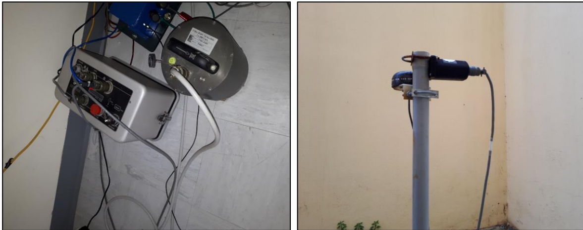
Figure 2.5 The ATEI SGM station, the REF TEK 130-SM as well as the CHAN Guralp seismometer(left) and their GPS antennas(right).
