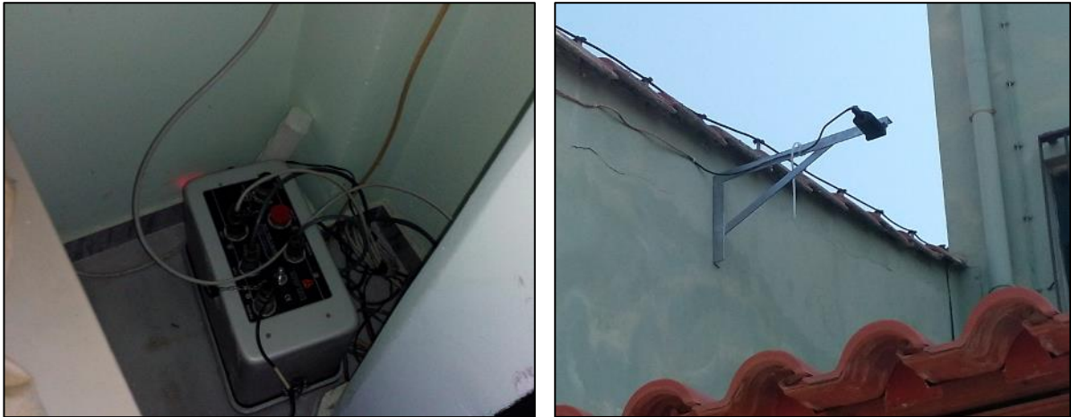
Figure 2.3 The ABEA station, the REF TEK 130-SM(left) and the GPS antenna (right)in the relative new high school building.
