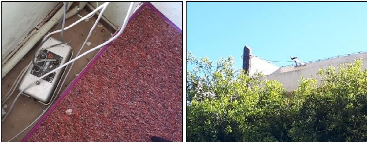
Figure 2.11 The MULT SGM station, the REF TEK 130-ANSS/02 and the GPS antenna
