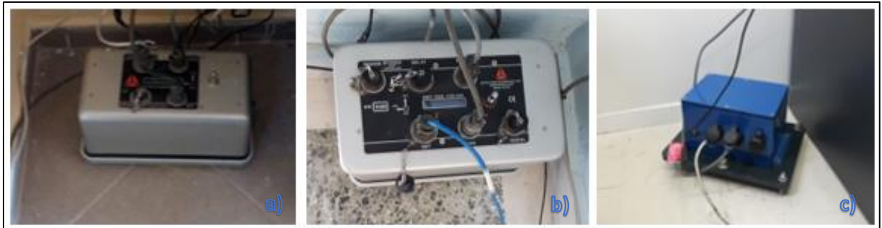
Figure 2.1 a, b, c. The three types of accelerometer installed for the SGM network, the Ref Tek 130 ANSS/02(left) the 130 SM (middle) and the GSense (right)
