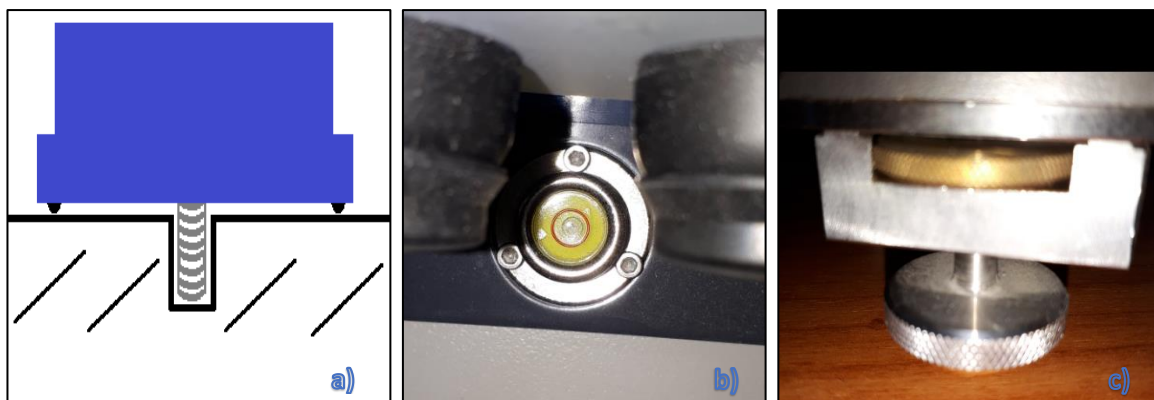
Figure 2.17 Securing the accelerometer to the ground through an anchor bolt (left) and the alignment blister (right) used for calibrating the sensor to be parallel with ground.
