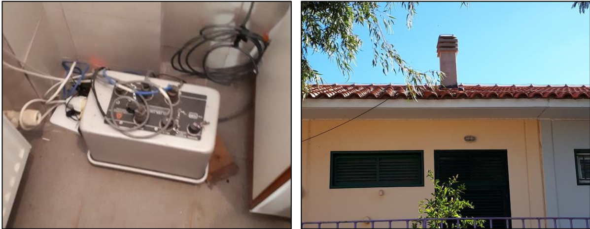
Figure 2.9 The LENT SGM station, the REF TEK 130-SM(left) and the GPS antenna(right).
