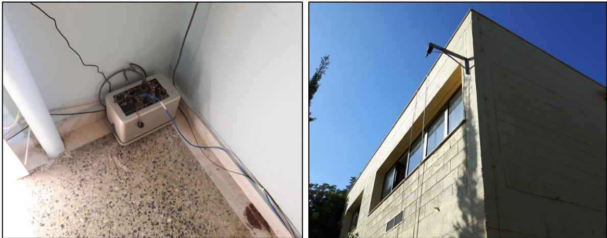
Figure 2.15 The POLY SGM station, the REF TEK 130-SM and the GPS antenna
