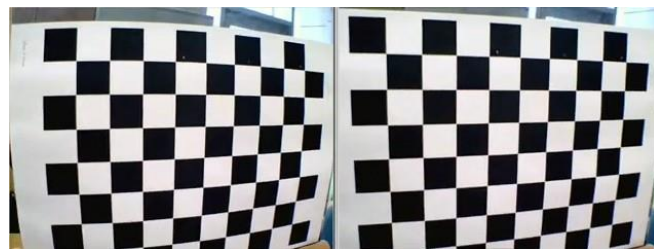
Fig 28. Camera calibration and distortion correction
