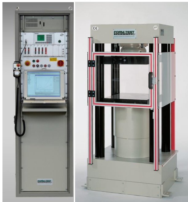
Figure 5.2: The uniaxial load testing machine (Form+Test ALPHA3-3000, 3000kNt), equipped with programmable digital control unit (AS C20 N).
