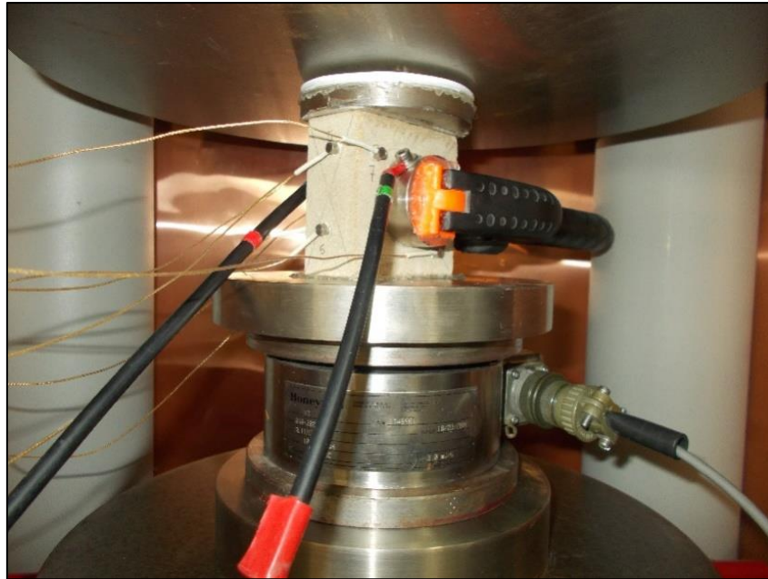
Figure 5.14: The prismatic sample inside the testing machine before the compression test.
