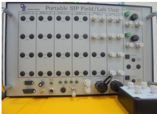
Figure A.1 Portable Field/Lab Spectral Induced Polarization (PSIP) instrument
