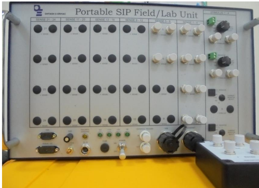
Figure 4.2 - Portable Field/Lab Spectral Induced Polarization (PSIP) instrument by Ontash company.
