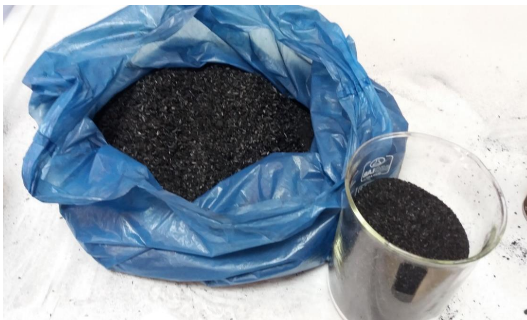
Figure 4.7 Biochar from blending of paper sludge and wheat husks that used in the measurements.
