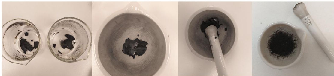
Figure 60 When graphite oxide has fully dried, it is transferred to a mortar to be pulverised with a pestle into a fine powder.
