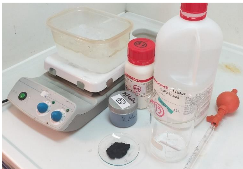
Figure 51 Experimental set up for preparation of graphite oxide via modified Hummers method. An ice bath and magnetic stirrer are needed. Sodium nitrate and potassium permanganate are added as oxidising agents in a mixture of graphite in sulfuric acid.
