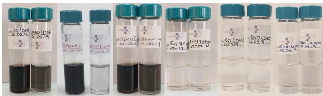
Figure 76 (From left to right) GO and RGO in DMF, DMSO, NMP, THF, DES.
