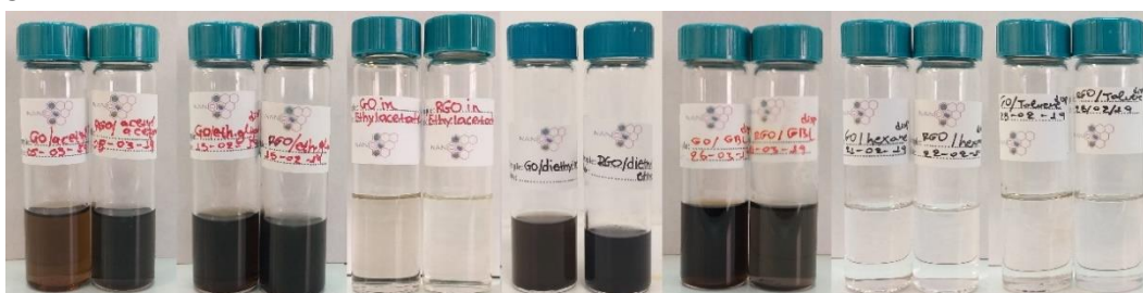
Figure 75 (From left to right) GO and RGO in AcAc, EG, EA, DETr, GBL, Hex, Tol.
