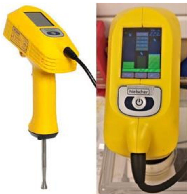
Figure 70 Left: Ultrasonic probe used for the preparation of GO and RGO dispersions (Image taken from reference 252) Right: Settings screen of ultrasonic probe. Power is set at 100W and frequency is set at 26 KHz.
