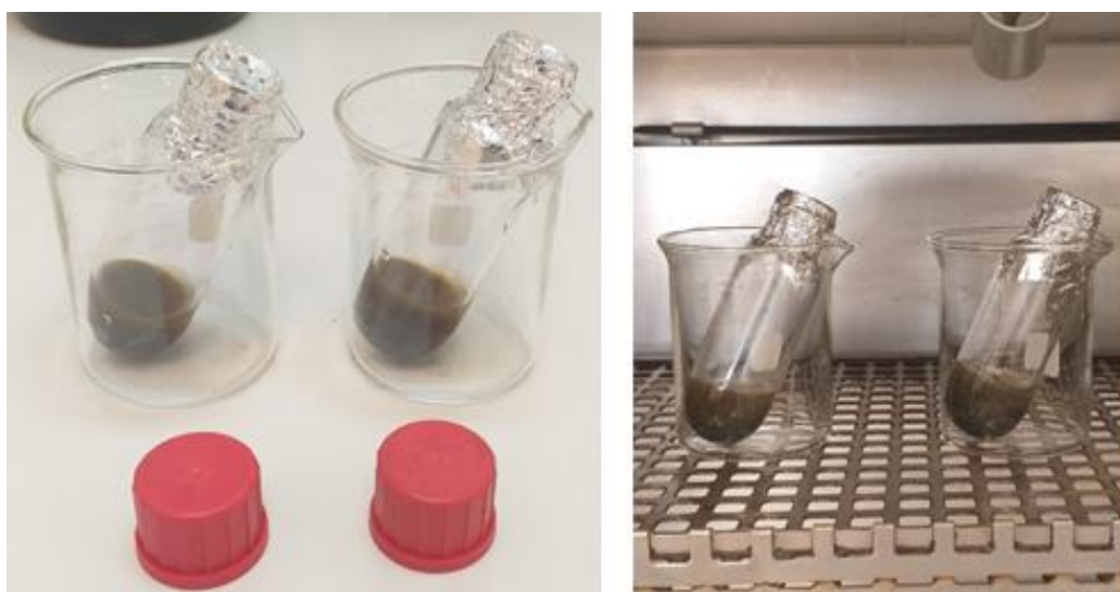
Figure 59 The washed graphite oxide is left to dry in an oven at 55°C for several days until it is completely dry.
