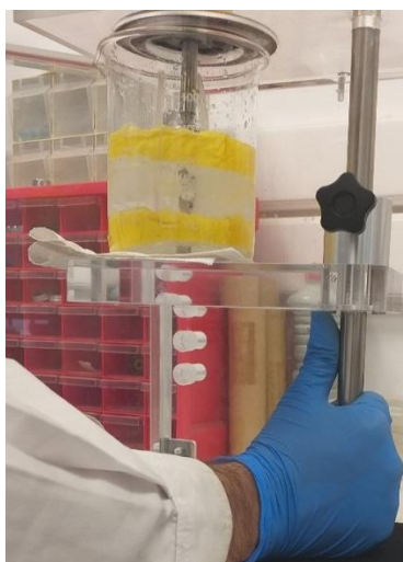
Figure 72 The ice bath sits on a shelf whose height can be adjusted to control how deep the ultrasonic probe is immersed.
