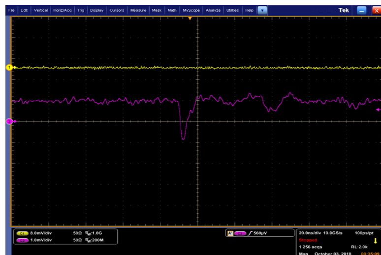
Fig.2.28 Dark current in the monitor of the oscilloscope before the recording of the harmonic signal
