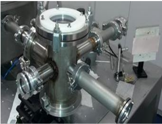
Fig.2.10 The chamber where HHG occurs.
